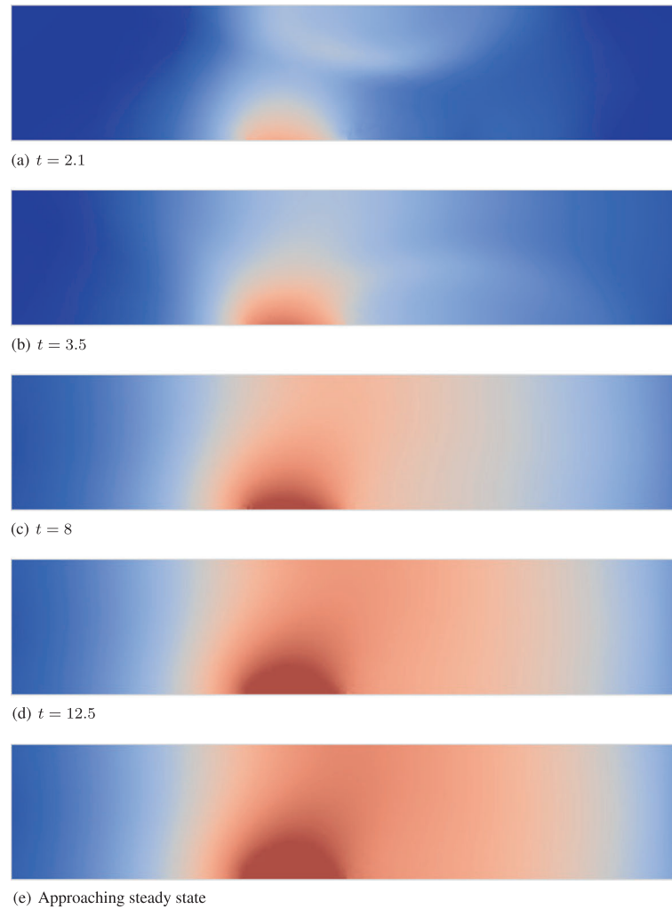
Figure 6. Subcritical Poisseuille flow: concentration solutions using linear color map for u \in [0, 0.01] with u = 0 \rightarrow blue, u \geq 0.01 \rightarrow red. (a) t=2.1 ; (b) t=3.3 ; (c) t=8 ; (d) t=12.5 ; (e) Approaching steady state.
